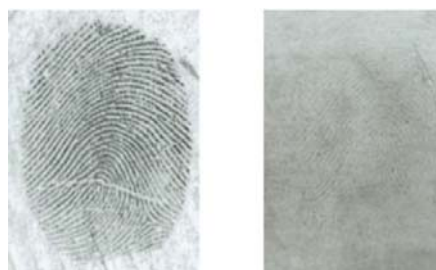
Figure 3. Latent fingerprints developed from matte screen protective films.
